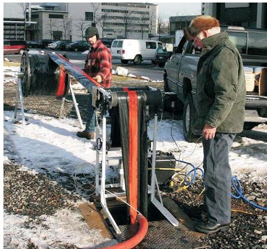
**2. Measure all significant flow paths at the same time with the Hydraulic Conductivity Profiler**
