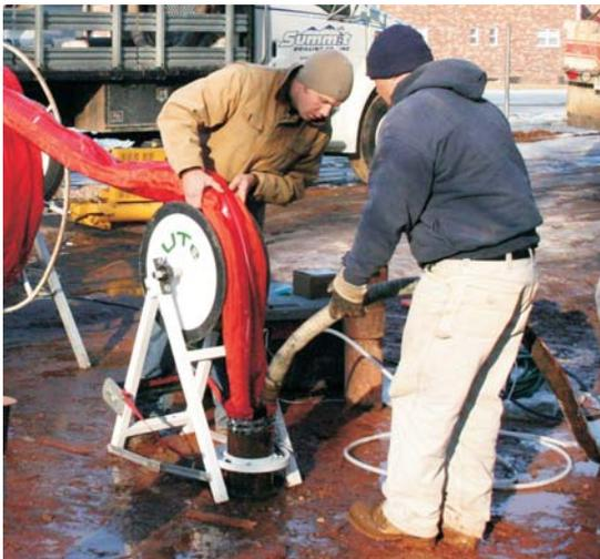
**3. Swap the sealing liner for a *Water FLUTE* multi level system. Measure the head profile and water quality profile, more easily than any other system.**
