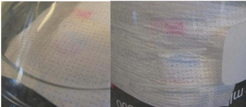
Figure 26: occurrence of faint staining after leaving a piece of FLUTE liner in PCE and TCE saturated solution
