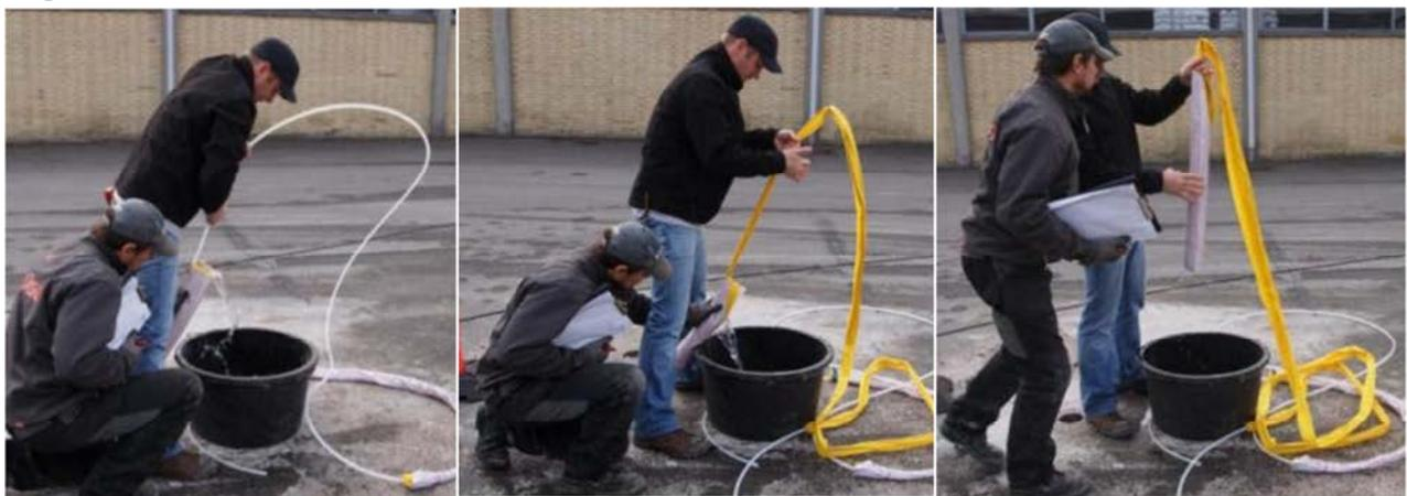
Figure 30: removal of FACT; left: pulling the tubing to invert liner & remove water filling; right: final recovery
