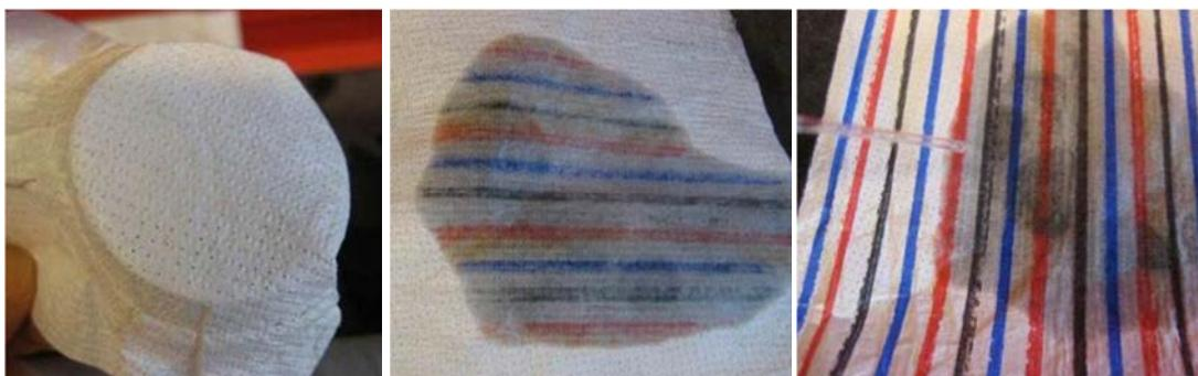
Figure 25: staining test results in PCE saturated air phase (left) and with DNAPL (middle and right)
