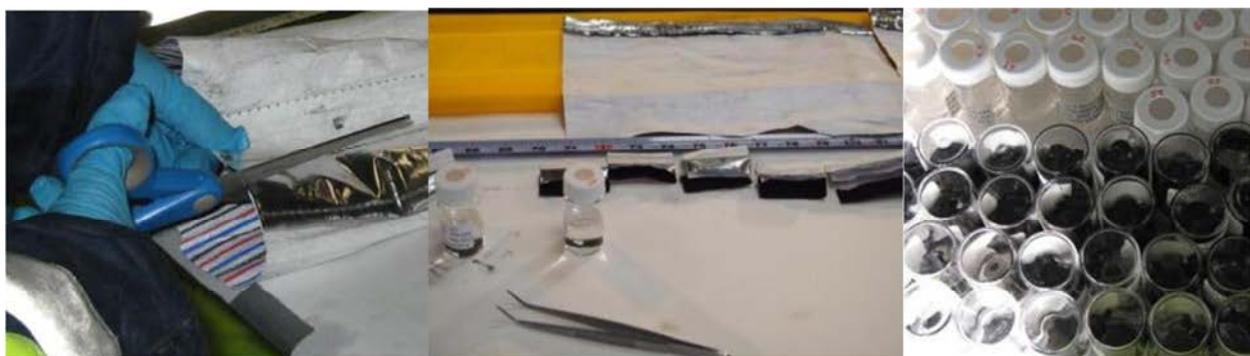
Figure 32: subsampling; right: cutting felt into half; middle: sampling of the carbon felt in smaller parts & 30 cm backup, left: vials filled with 10ml water and sample
