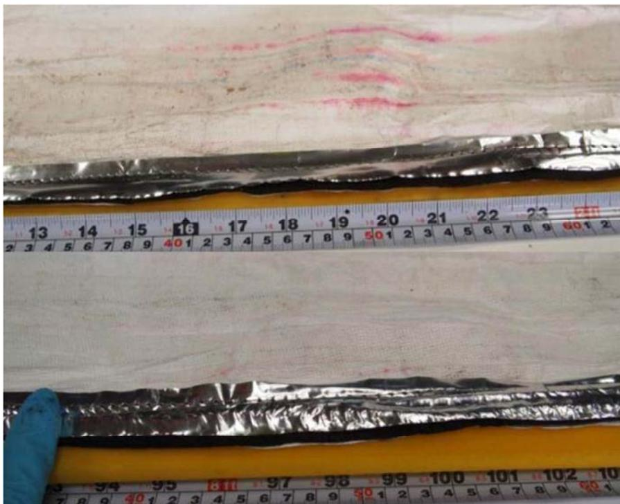
Figure 38: Flute CTF 3 small, mainly red staining at around 50cm (upper) and very light staining at around 2.5 m (lower)
