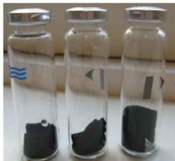
Figure 12: direct analysis of carbon felt in GC headspace vials
