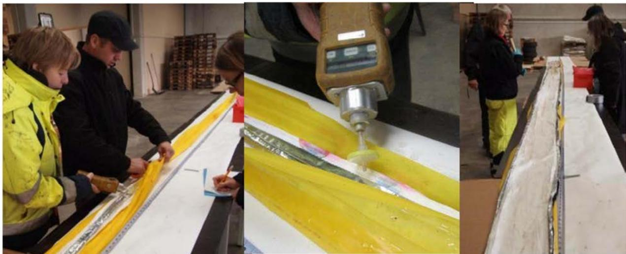
Figure 31: sampling; left and middle: opening of liner and PID measurement, right: examination of staining
