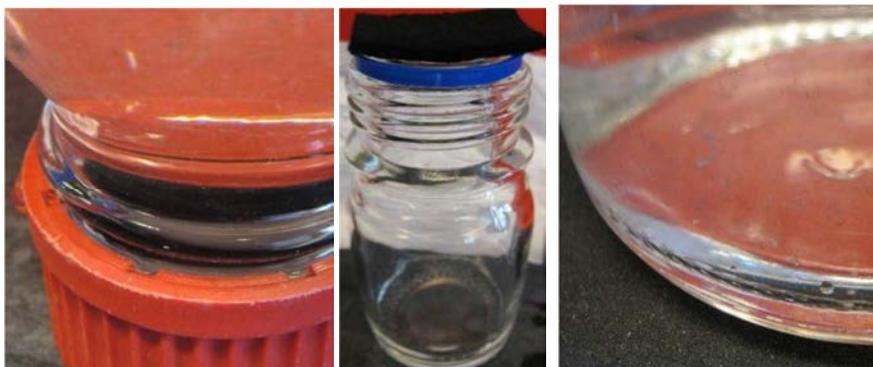
Figure 18: adsorption under DNAPL contact with carbon felt in lid (left), adsorption of saturated air (middle) and in saturated aqueous PCE solution with PCE drop
