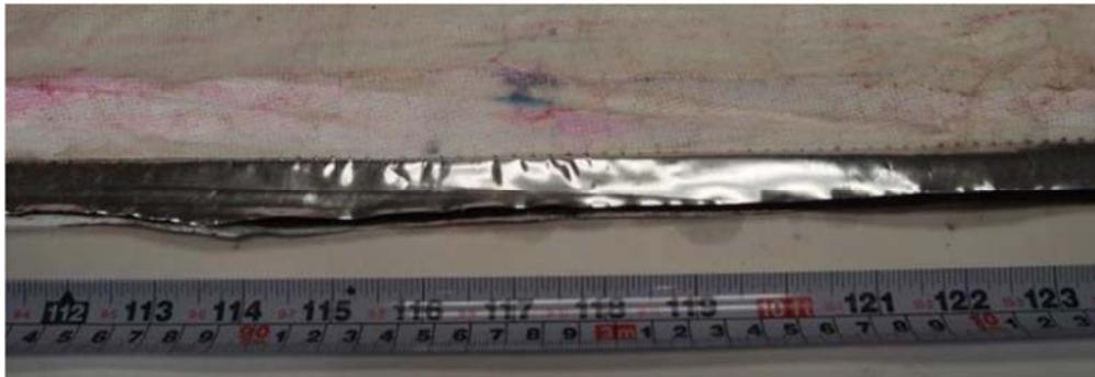
Figure 37: CF2 staining around 3 m b.s.
