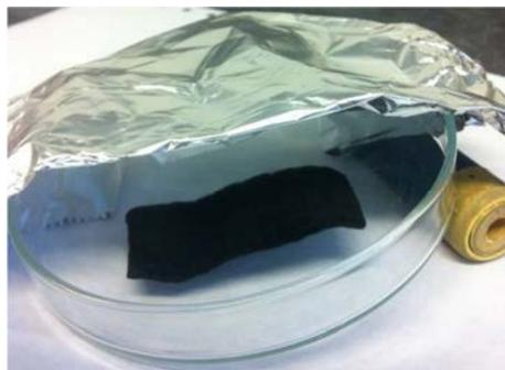
Figure 15: carbon felt left for volatilization in a Petri glass covered with aluminum foil to avoid ventilation
