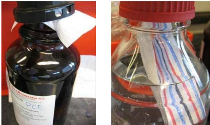
Figure 17: FLUTE liner material exposed to PCE saturated air & aqu. saturated PCE/TCE to examine staining
