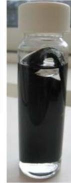
Figure 16: arrangement of 30cm carbon felt in 40ml vial
