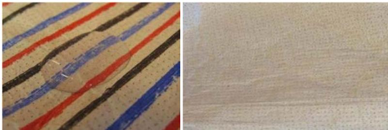
Figure 24: instantaneous staining test with drop of saturated aqueous PCE (left) → effect: no staining (right)
