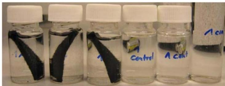
Figure 14: adsorption setup with 3 carbon felts exposed to a certain PCE solution and 3 control vials without carbon felt for determination of the initial concentration and compensation of “losses” due to volatilization
