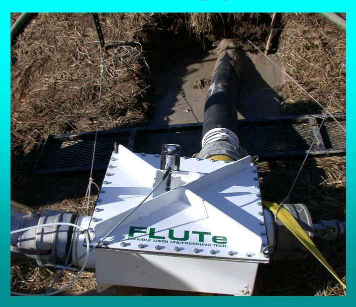
The liner is deployed from a large canister via a 90 deg. elbow
