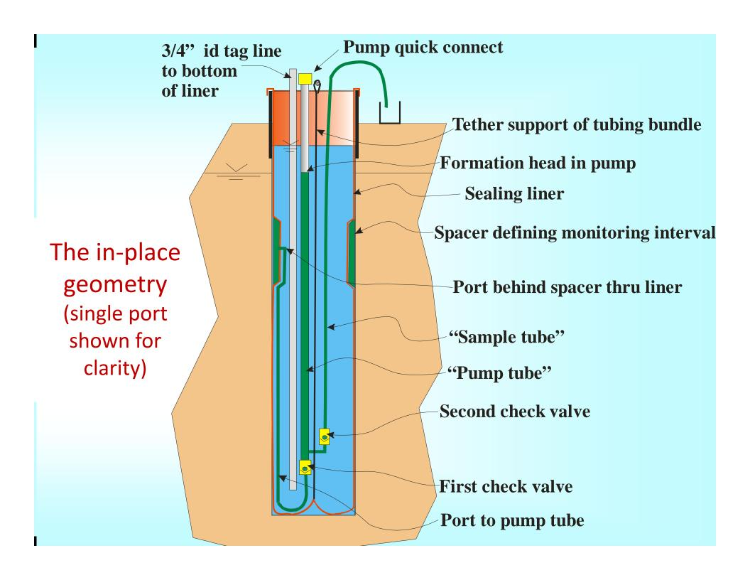
The pumping procedure 2 purge strokes 1 sample stroke
