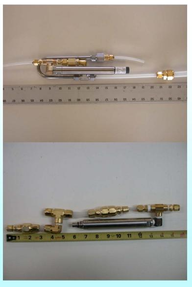
Old pump of stainless tubing, side access for first check valve, smaller valves.
