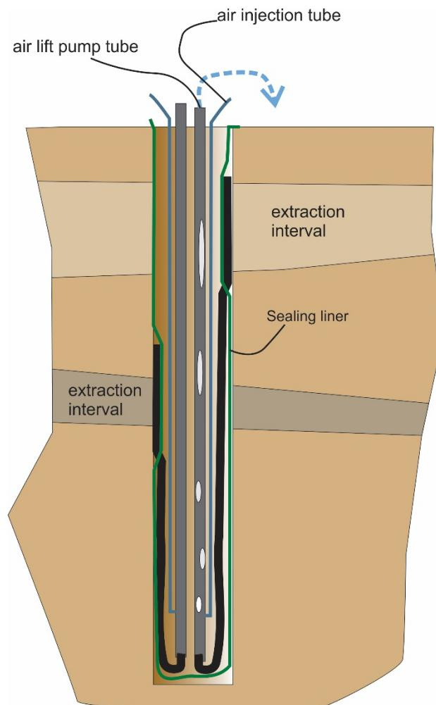
Figure 1. The DEIL geometry showing the large tube from the extraction interval and the larger air lift pump tube. Air injected near the bottom of the pump tube reduces the density of the water column and causes it to be driven to the surface. Water table depth at the port should be less than half the liner depth.
