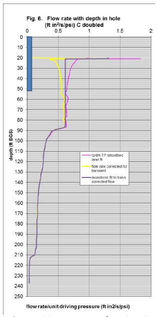
Fig. 7. Flow rate with depth in hole (ft in<sup>2</sup>/s/psi) S/5 0.5 1.5 Q/dH-TP smoothed over N flow rate corrected for monotonic ft to trans corrected flow flow rate/unit driving pressure (ft in2/s/psi)
