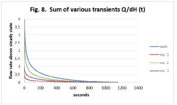
different rock type and transmissive interval, the above correction is not exact. However, it is interesting that the sum of many different transients as shown in Fig. 8 still looks like a transient with the same asymptotic decay.
